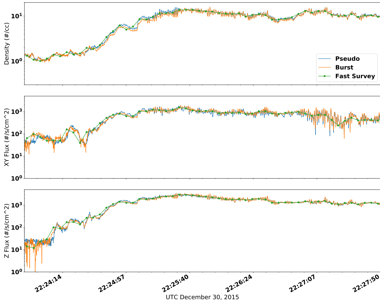
Figure 4.13: December 30, 2015 (MMS1); Ion pseudo moments (blue) compared to level 2 burst resolution data (orange) and fast survey (green). From top: spin plane (XY) flux, spin aligned (Z) flux, number density.
